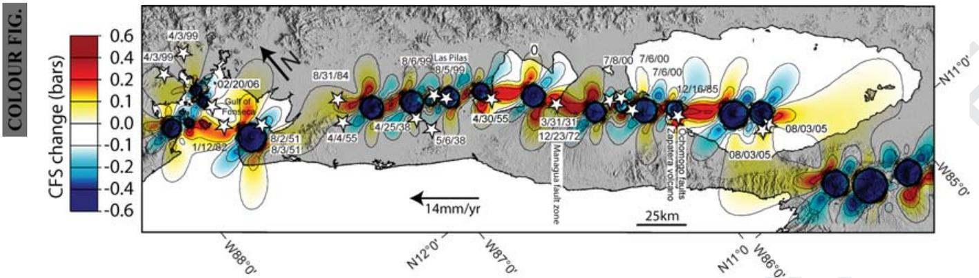
**Figure 4.** Coulomb stress changes on  $N40^{\circ}E$  oriented left-lateral fault planes in Nicaragua, showing maximum between volcanoes and minimum at volcanoes. The shear and normal stresses caused by regional shearing without a weak zone are 1.5 and 0 bars. The contour interval is 0.1 bars.
