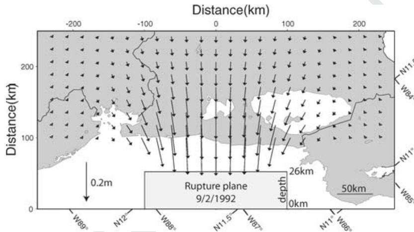
**Figure 5.** Displacement field resulting from the 1992 subduction earthquake. The rectangle indicates the slipping patch, 200 km long and 100 km wide with a  $15^{\circ}$  fault dip and 0.5 m slip inferred from the aftershocks (Ide *et al.* 1993).
