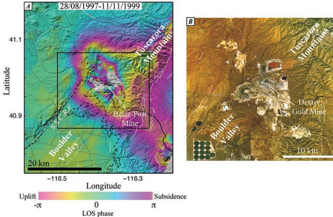
**Figure 3.** Bedrock subsidence (a) 2 years interferogram of the bedrock subsidence in Tuscarora mountain over shaded relief of topography. Southern Sheep Creek Range Fault (S.S.C.R.F.). Faults (white lines), main roads (grey lines), bedrock-sediment limit (dashed black line). (b) Landsat image of the Dexter Mine complex.
